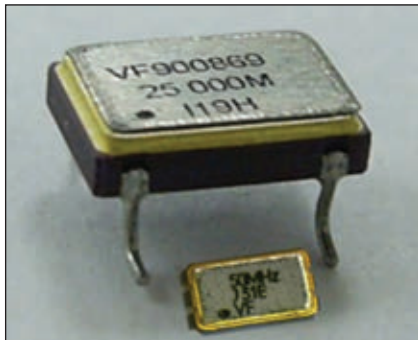
▲ Fig. 2 Valpey Fisher VFH3225 package compared to traditional 7 × 5 mm package.
